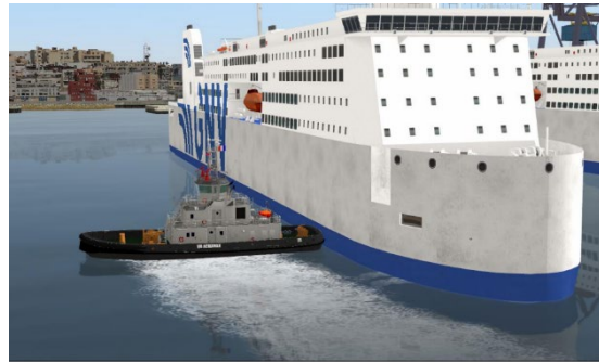
Tug pushing a 203 m long ferry from the starboard bow
