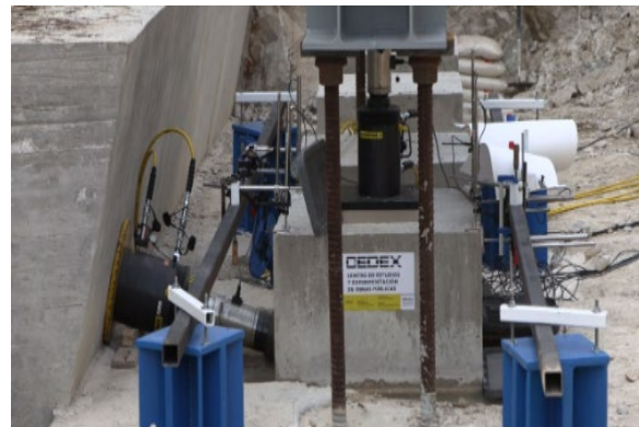
Setting up an in situ shear test for one of the cubes. Side view
