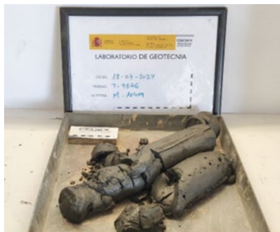
Material extracted from one of the Shelby tubes received at the Geotechnical Laboratory for testing.
