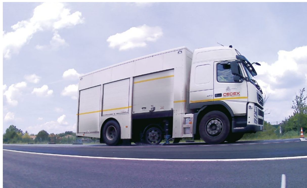
SCRIM device measuring the sideways force coefficient (SFC) of the pavement.
