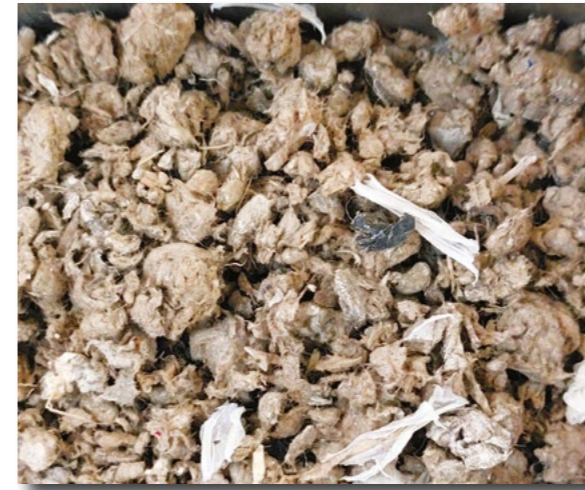
Mixed cellulose-polymeric waste used in an SMA mix.
