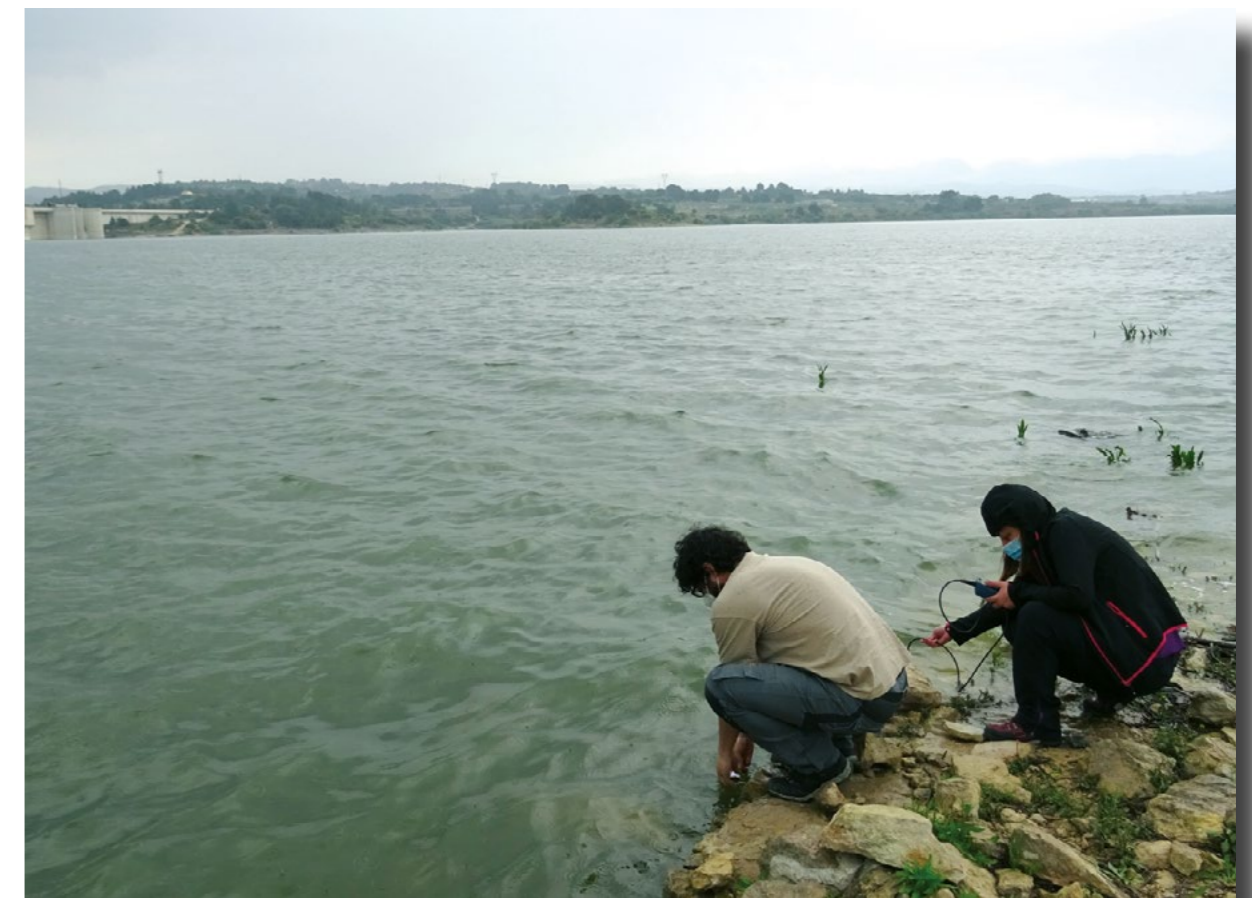
Measurement of unstable parameters in a water sampling campaign for isotopic study of water tightness of the Bellús reservoir.
