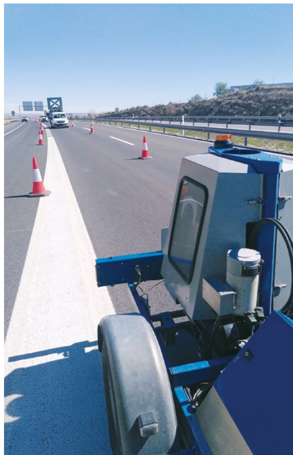
Testing by CEDEX FWD for the verification of indicator 4. Highway A-2 concession, in the province of Zaragoza.
