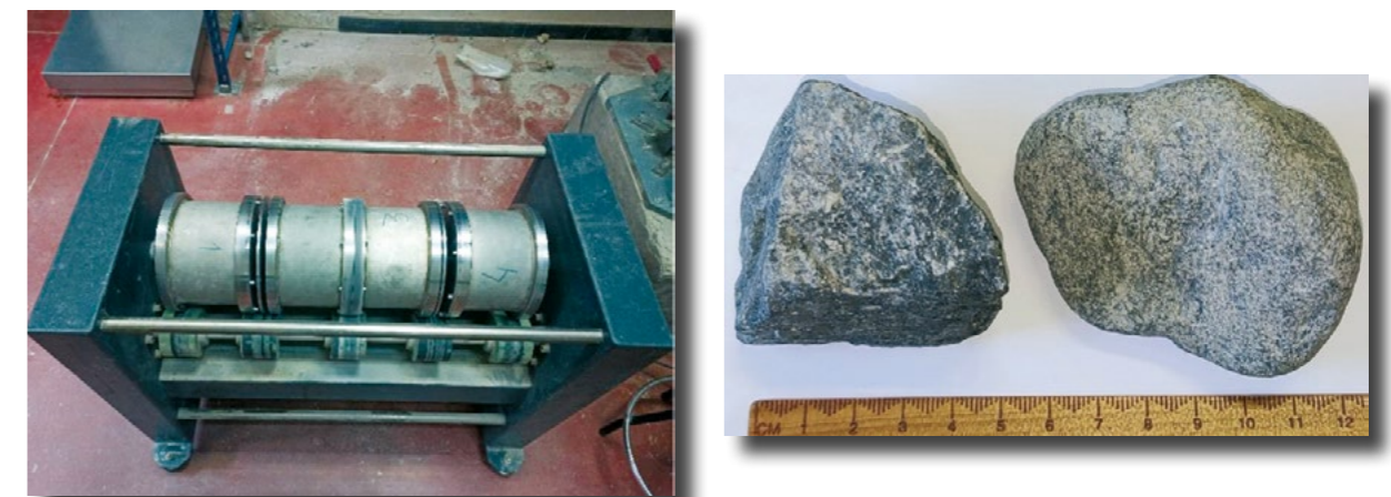
Figure 3. LG-CEDEX Micro Deval equipment used for ballast degradation studies.
