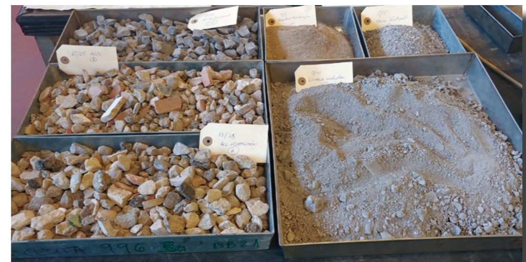
CDW aggregates and USW incineration slags for concrete production.
