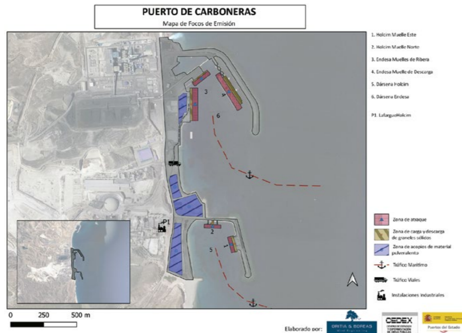
Schematic plan of sources of emission from docks, industrial activities and land transport of the port of Carboneras.
