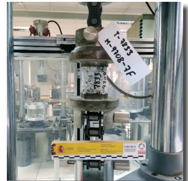
Direct tensile test on a low slenderness granite specimen.
