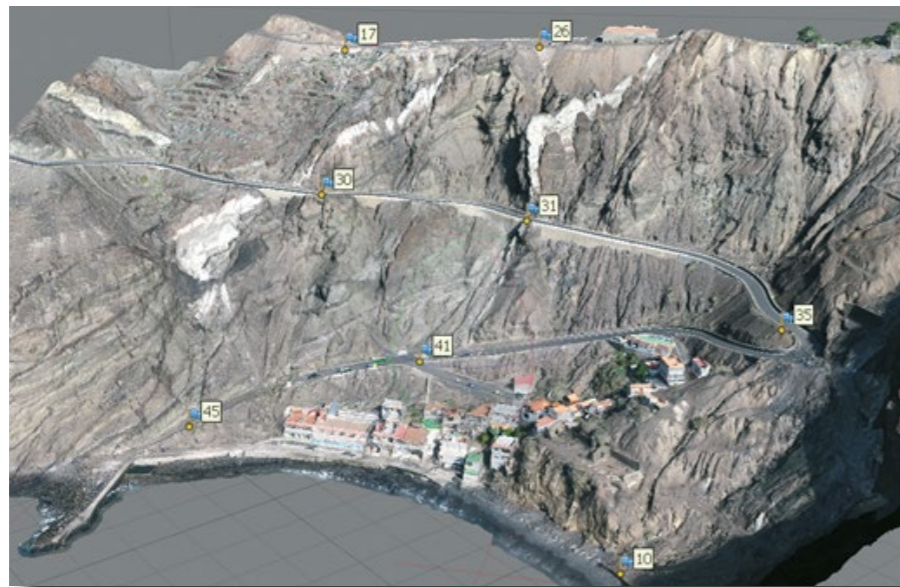
Figure 1. Digital terrain model produced from drone photogrammetry.
