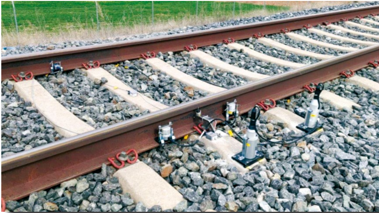
Figure 4. View of the instrumentation mounted on a section of the Madrid-Barcelona high-speed line.
