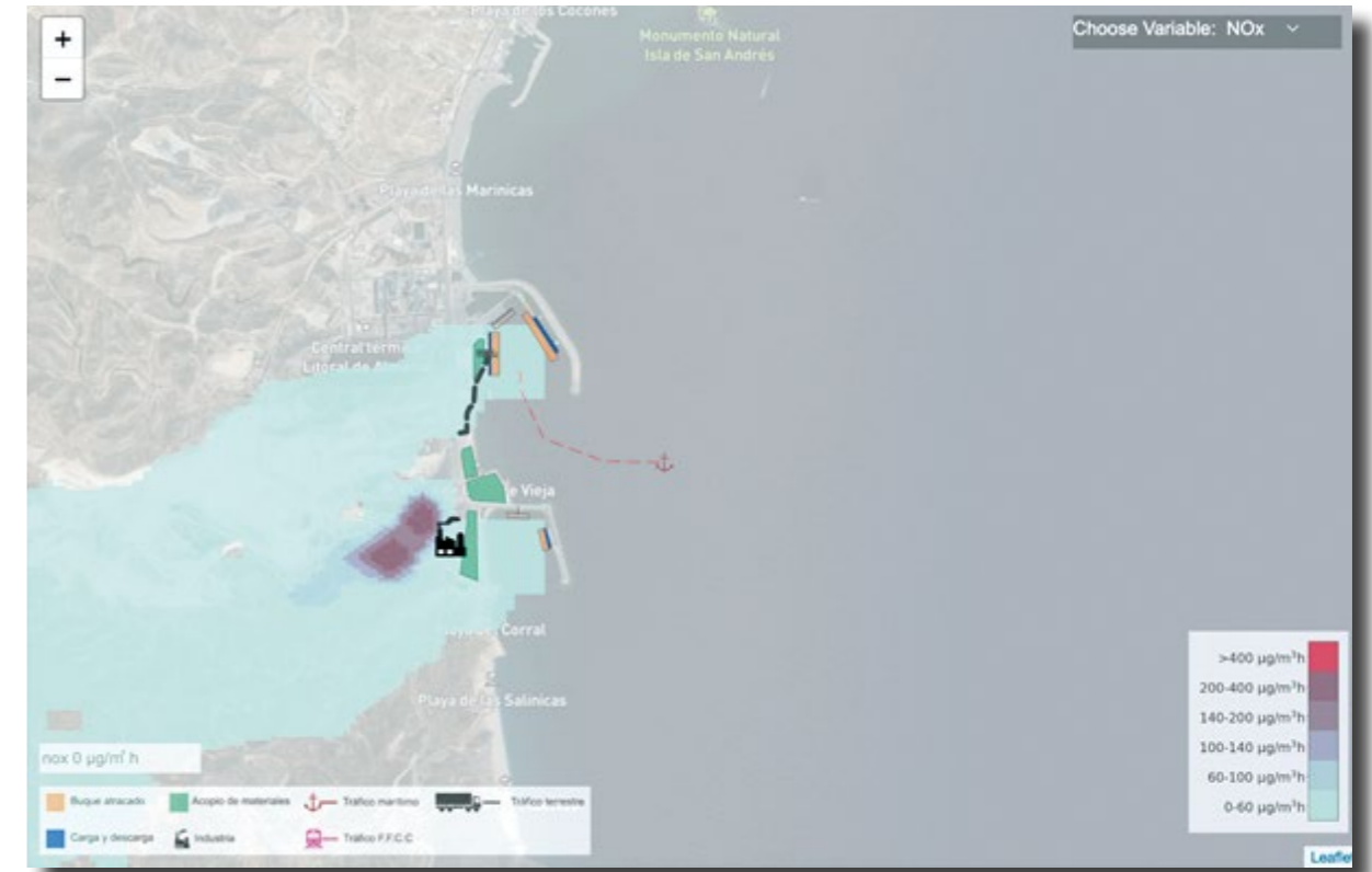
Simulation of dispersion of pollutants (NOx) in one day of operation.
