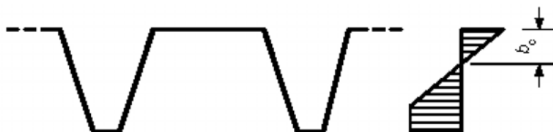
Figure 73.11.1 Plastic distribution stresses in the portion in tension
