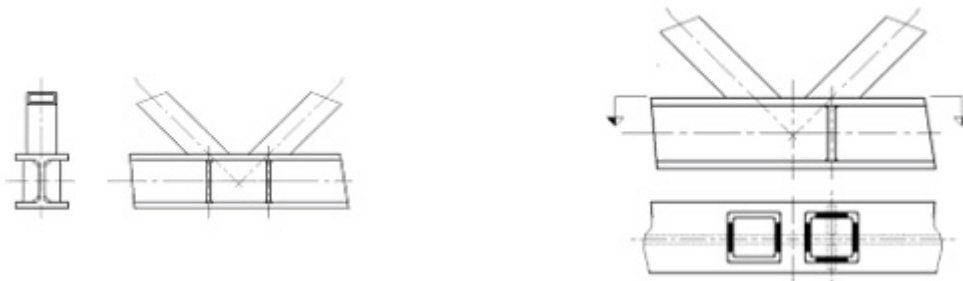
Figure 64.8 Effective perimeter of the diagonal or upright without (left) and with (right) stiffeners
